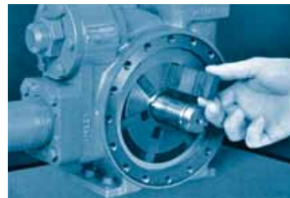
Simple vane replacement requires no special tools.
